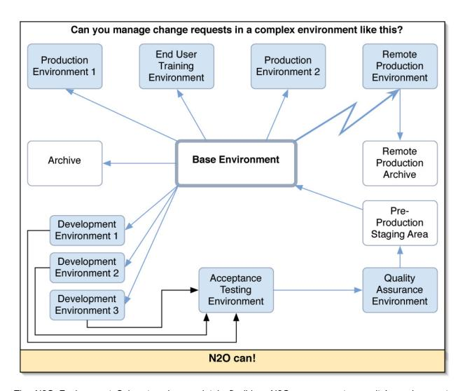
The N2O Environment Subsystem is completely flexible. N2O can support any site's environment, including complex environments like the one shown above. N2O can support multiple development, test, production, and other environments. If a site's environment setup changes, N2O will change with it. New environments can be added quickly, and obsolete environments can be removed easily.
